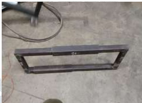
Figure 4. Guide Column for Lifting
