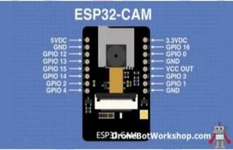
Figure 2.2: ESP32 camera pinout
