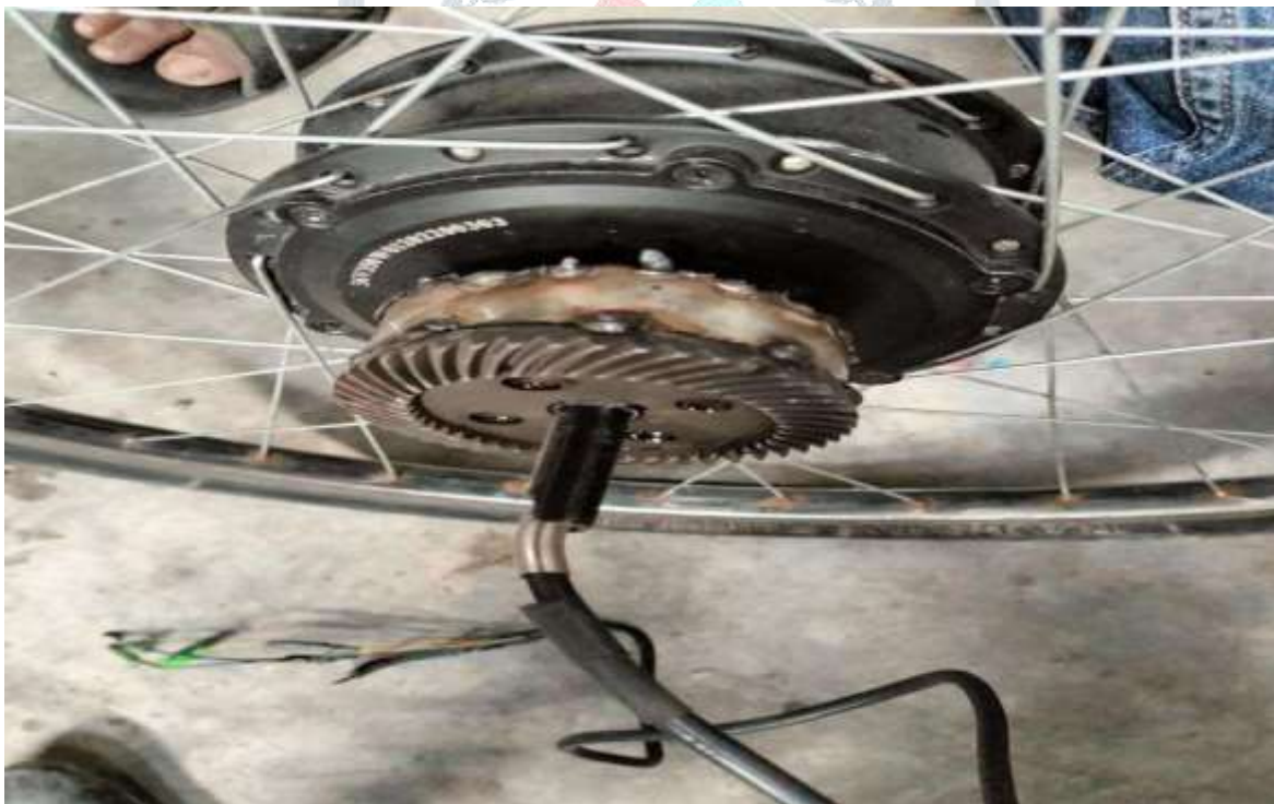
Fig 10: Fabricated Hub Motor and Gear on Rear Wheel
