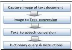
Smart Reader initially takes a picture of the text document. Open CV is used to take a picture of a book page and use the built-in pre-processing tools. Therefore, the image will be in the best possible condition for the OCR module to transform it to text. This will revolve around the concept of picture processing. The time is better now to outline it.
