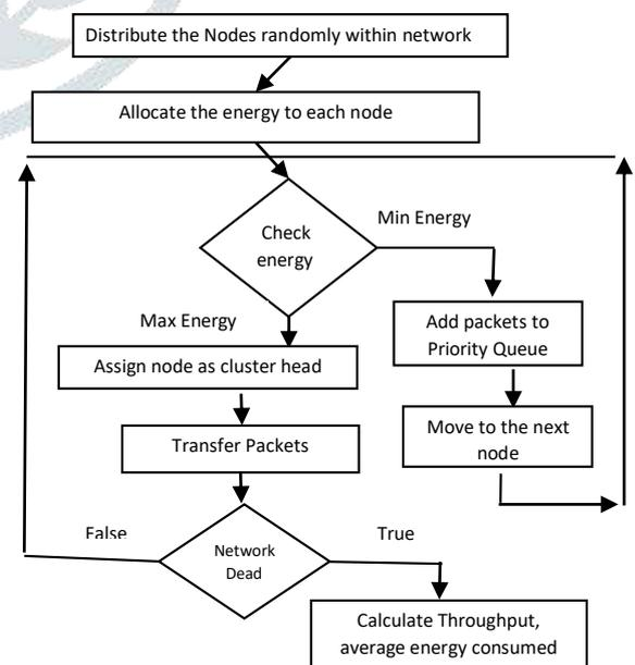
Figure 2: Structure of proposed methodology
