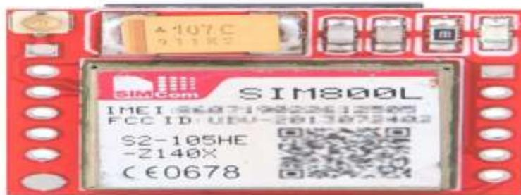
**Powering up :** The SIM800L is powered up by providing a voltage supply of 3.4V to 4.5V to the VCC pin. Once powered up, the module performs a self-check and initializes itself.
