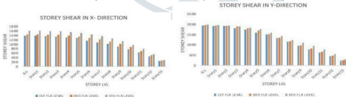
Figure 7.1 Maximum storey shear in direction of X Figure 7.2 Maximum storey shear in direction of Y
