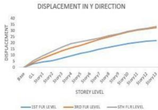
Figure 8.4 Joint displacement in direction of Y
