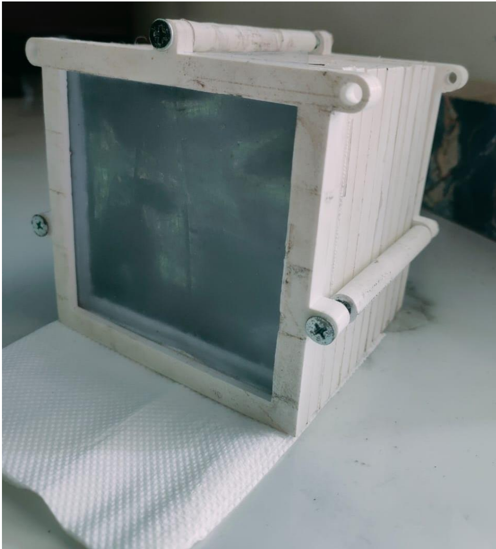
Fig 1d Experimental setup of 10 stage multilevel solar still
