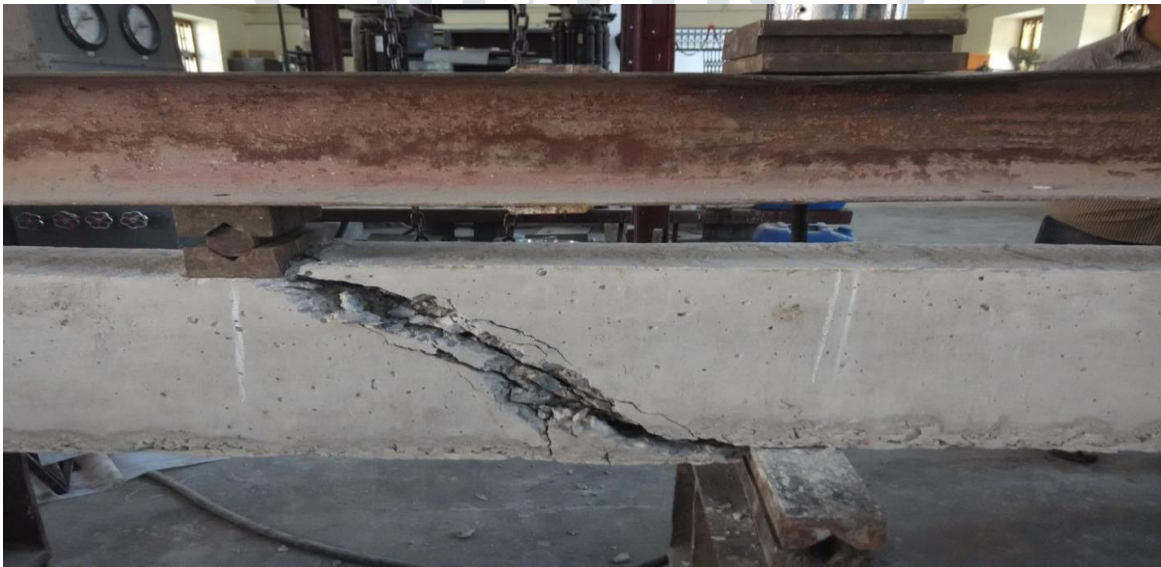
Fig 3.4 Ultimate Failure of the Beam
