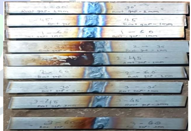
Fig. 5: Specimen After welding
