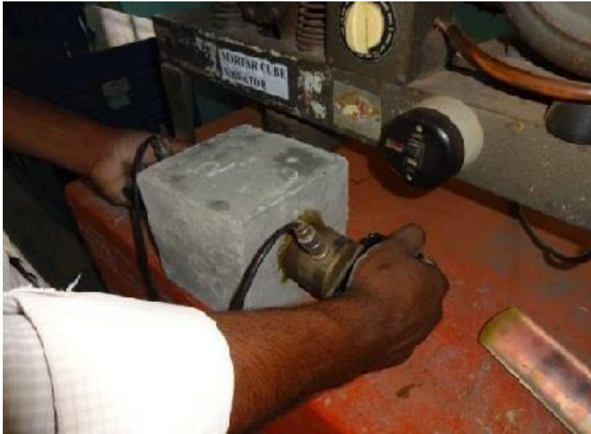
Figure 2.5 UPV test on CS concrete specimen
