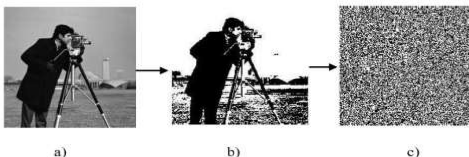
Figure 4. Image conversion (From original image to LSB image) a) Original image, b) Grey scale image, c) LSB image
