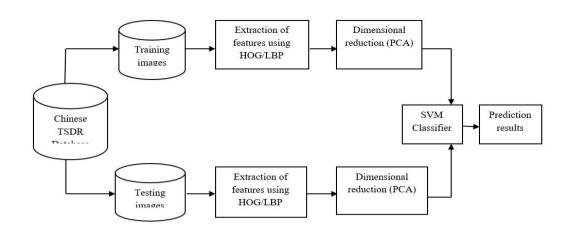
Schematic diagram of the proposed method for TSR
