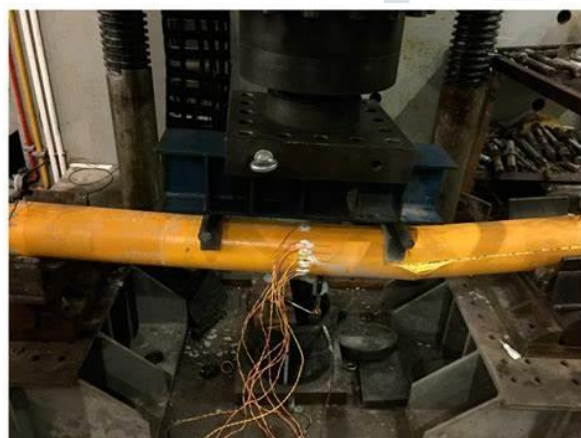
Bending of concrete filled steel tubes
