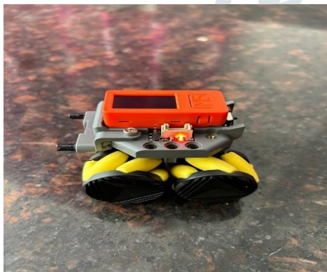
Fig.3. Rover When interfaced with M5 Stick C Plus
