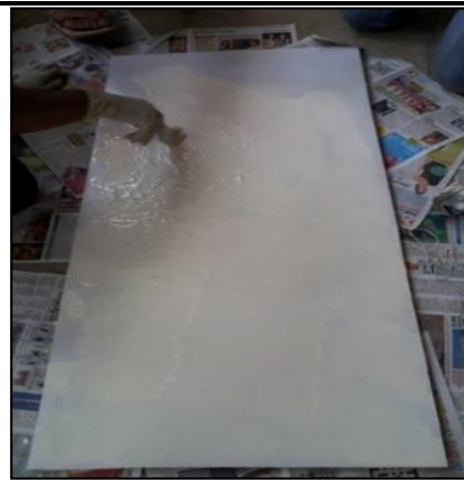
(c) Gel coat applied to mold and planks
