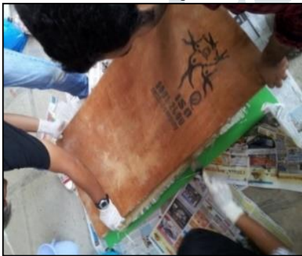
(f) Wooden plank used to support the mold.
