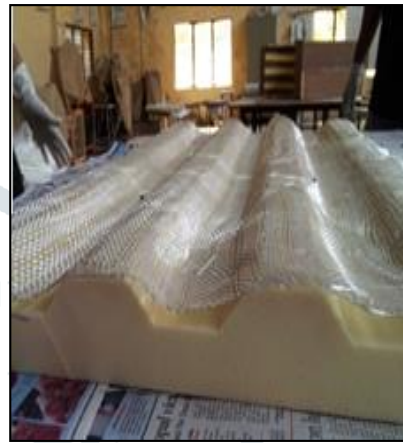
(e) Fiber glass placed on the PU foam core
