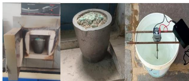
Figure 2. Experimental procedure of synthetic zeolite
