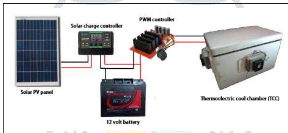
Fig. 2.1. Schematic of components assembly of developed thermoelectric cool chamber
