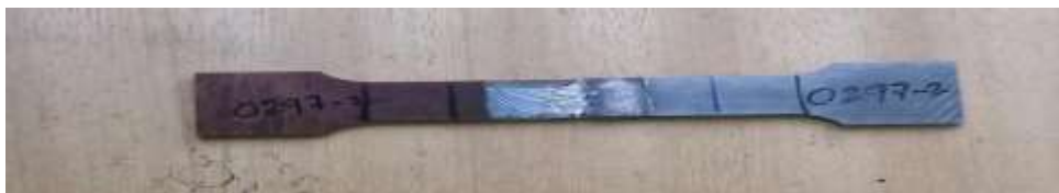
SAMPLE COLLECTED FROM HEXAGONAL PROBE WELDED AREA FOR MEASURING OF WELDING STRENGTH
