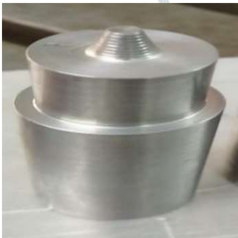
SAMPLE COLLECTED BY CYLINDRICAL PROBE FROM WELDED AREA FOR MEASURING OF WELDING STRENGTH
