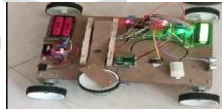
Fig 15: Implemented Automatic irrigation system using arduino
