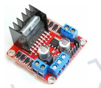
Motor driver L298N: A dual H-bridge motor driver module, which can offer two-way control of two DC motors with high current carrying capacity.
