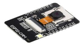
ESP32 CAM module can be identified as a smallboard that interfaces the ESP32 microcontroller with a camera, thus enabling WiFi connectivity as picture and video recording functions.
