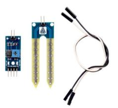
The soil moisture sensor is one of the sensors that are often employed in agriculture or automatic irrigation to measure the amount of water held in the soil.
