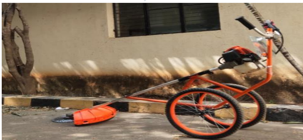
Fig1: Development of agriculture weeder operated by 2- stroke petrol engine
