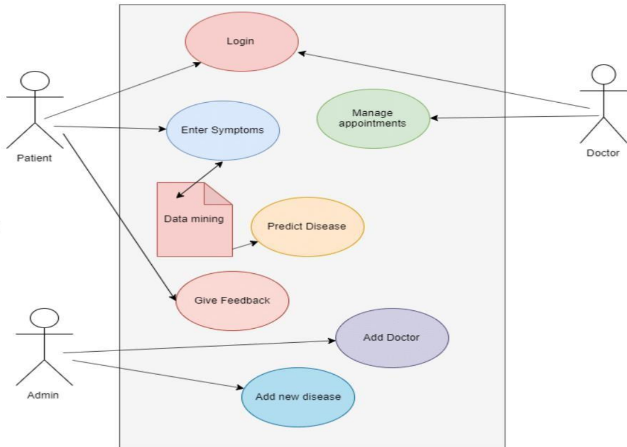
Figure 7.1: Use Case diagram of System The use case diagram shows the actors of the system and various tasks performed by them in the system.
