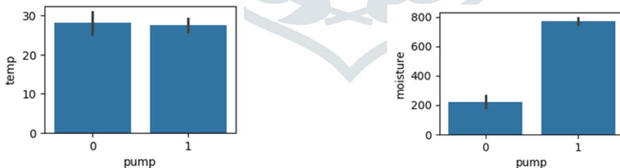
Fig. No. 5.3. Showing mean moisture and temperature when the pump is either on or off
