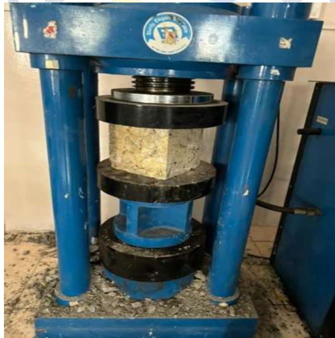
Fig: Cube placed for testing in compression testing machine
