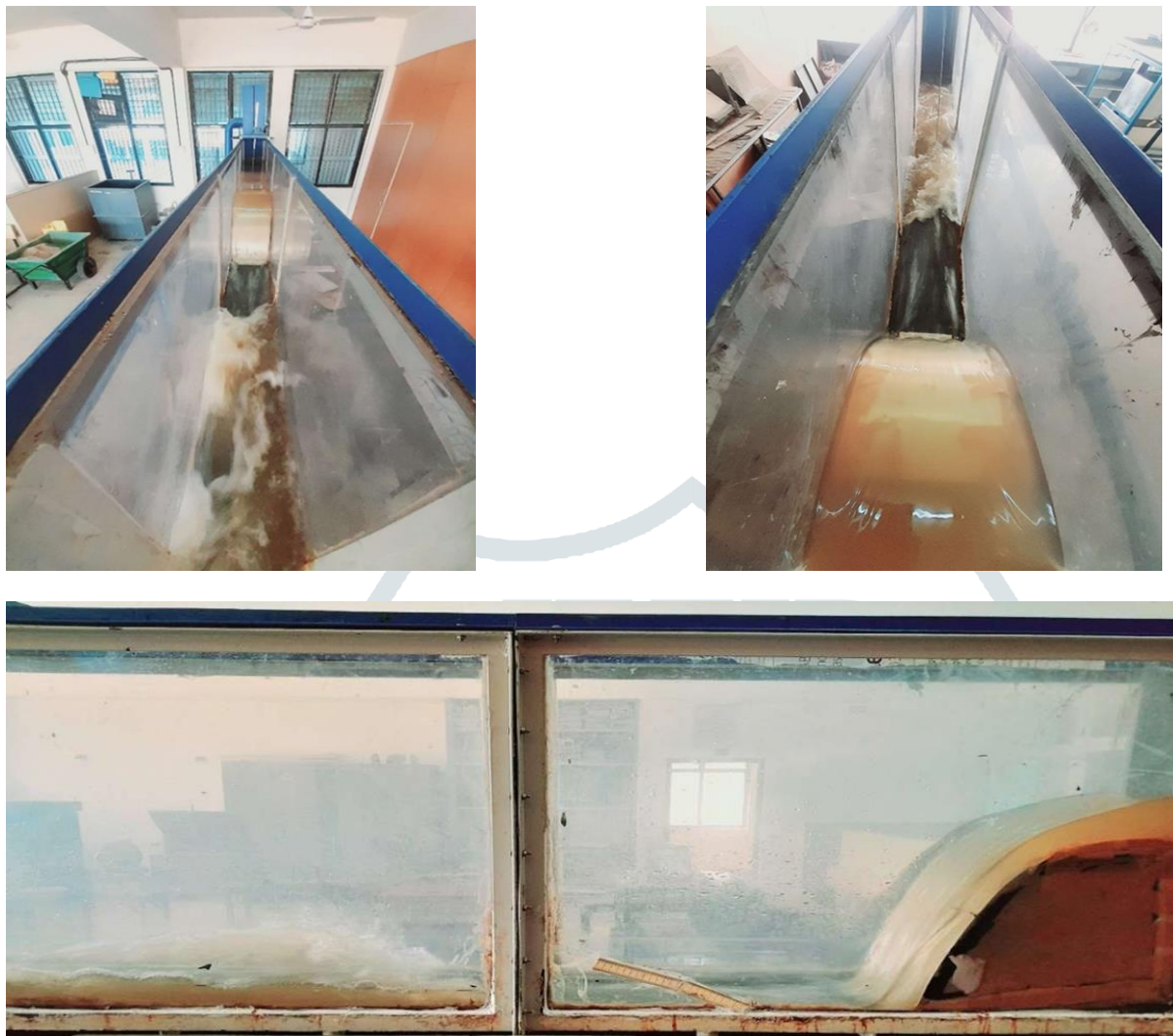
Figure 1. 4 Image of Hydraulic Jump Formation
