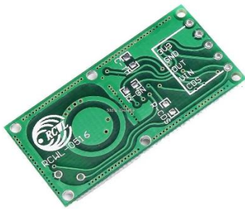
Fig - RCWL-0516 Microwave Radar Sensor
