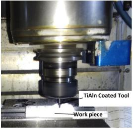
Fig. 1: Milling setup
