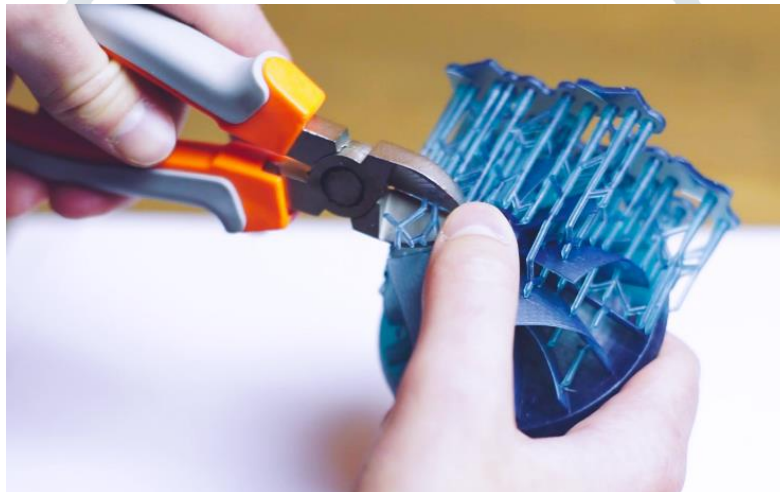
Photo. 2 Support being removed from a model with metallic tool (Courtesy - 3D Hub)
