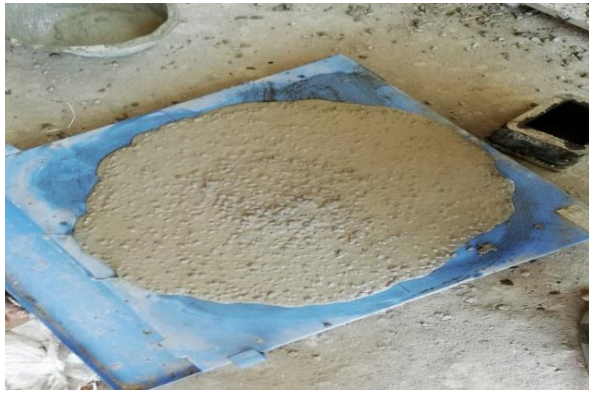
Fig (1): Slump flow
