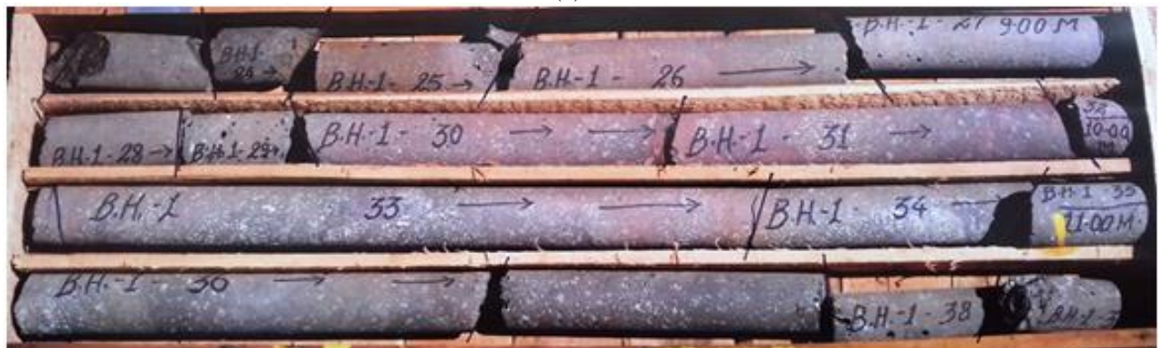
(b) Sample Bore Log for depth 8.0 to 12.0 m
