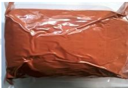
Fig.1: \text{Cu}_2\text{O} Nano-particles synthesized through precipitation method
