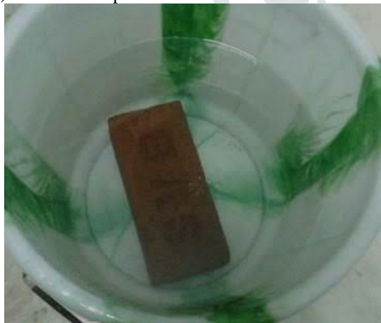
Fig. 6 Water Absorption test on brick
