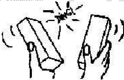
Fig. 7 Soundness test conducted by using two bricks
