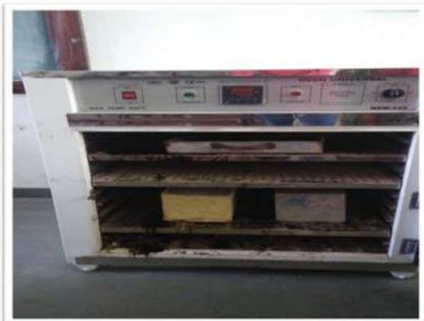
Fig. 5- Cube kept in oven at 200°C for 1Hr and 2Hr
