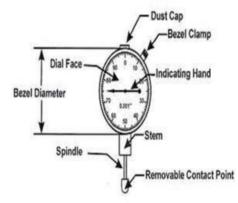
Fig 3: Specifications of dial gauge<sup>[5]</sup>
