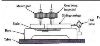
Fig. 1: Experimental setup of Parkinson's Gear Tester<sup>[1]</sup>
