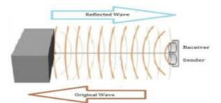
Fig-1: Ultrasonic sensor operations
