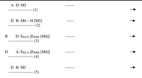
E<sub>KRB</sub> [M6] is Digital Signature calculated by Receiver B and sent to Sender A via Server D.
