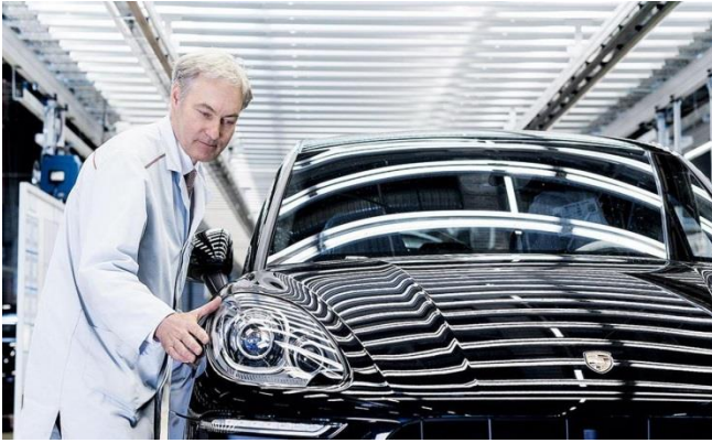
Fig. 2. inspection in light tunnel
