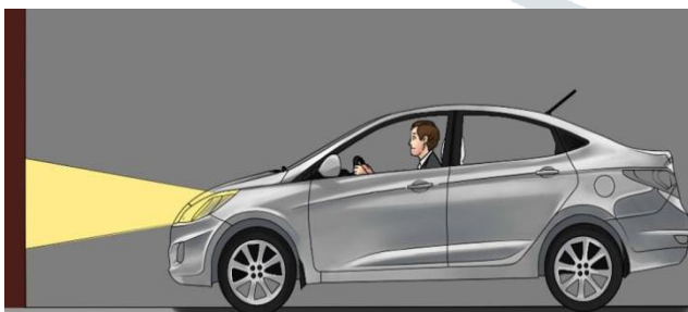
Fig. 1.(a) Headlight aiming using wall
