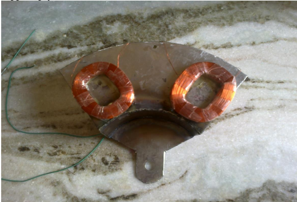
Figure 2 Actual photograph of Stator Coil
