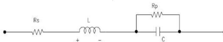
Fig. 3 First order circuit model of Supercapacitor
