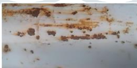
Fig 3.2 image of corrosion captured through camera [3]
