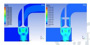
Velocity contours for conventional valve and modified Valve respectively.
