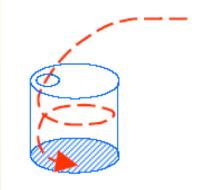
Turbulence is necessary to break the frame front into pieces so that each and every part of combustion chamber gets flame to ignite homogeneous air fuel mixture. If there is uneven flame distribution then there is incomplete combustion which gives less torque and also causes pollution.
