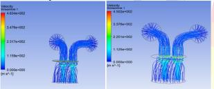
Velocity Streamlines for conventional valve and modified valve respectively.
