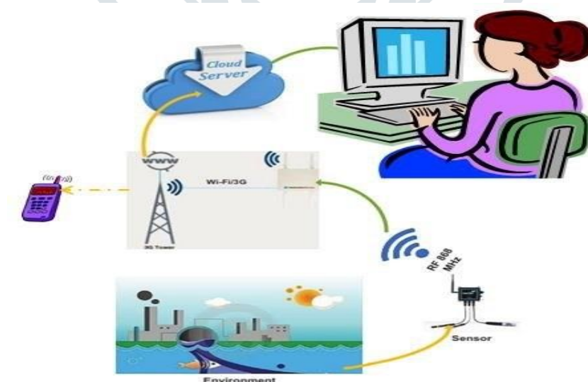
Figure 1: Basic Idea of IoT based Water Quality Analysis System
