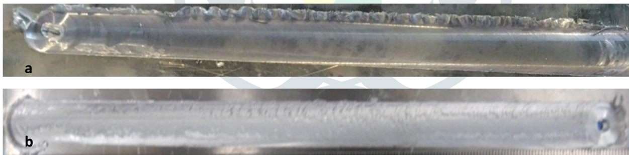
Fig 2. Surface appearances of the welded plates by a) Simple Cylindrical tool b) Square tool
