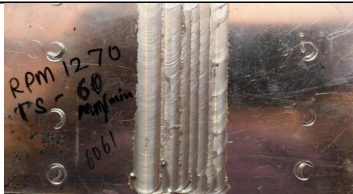
Fig. 2 Multi pass Friction Stir Processed Sample
