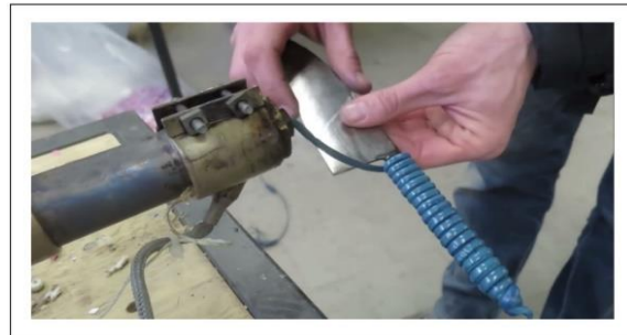
Figure 5 Safety Handle for Knife [1]
