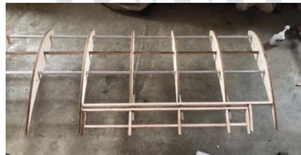
Fig.12. Aileron attached to the wing by 'pivot and round' hinges
