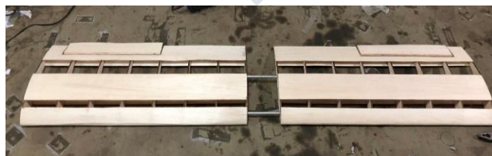
Fig.13. Wing masked with 1 mm thick balsa
