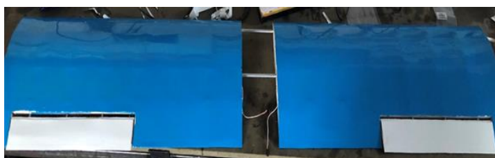
Fig.14. Wing covered with heat shrinkable adhesive covering film
