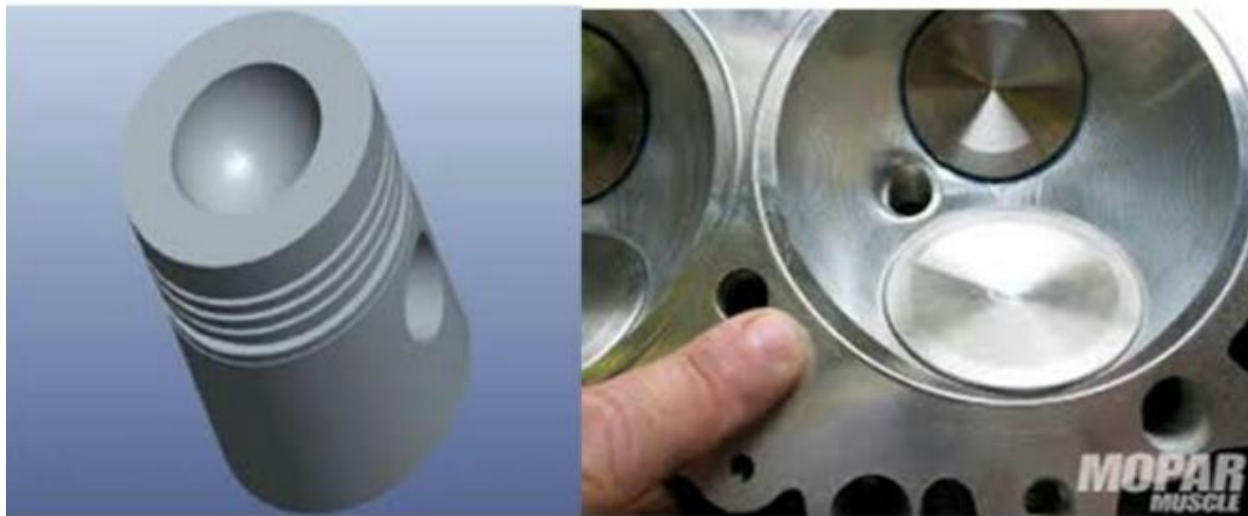
a) Fig 2 (a) Hemispherical Combustion Chambers. (b) Piston crown in Cylinder head
