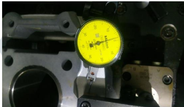
Fig. 8 Dial gauge indicator mounted on fixture
