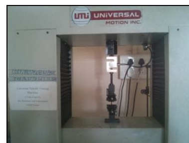
Fig. 05 UTM setup for Tensile Test
