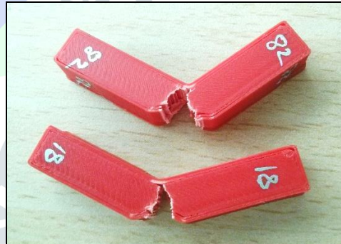
Fig. 11 Impact tested sample (partially broken)
