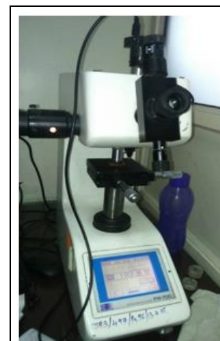
Fig. 16 Micro Hardness Measurement Test setup
