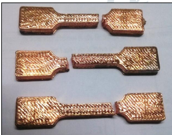
Fig 19 Samples broke after tensile test
