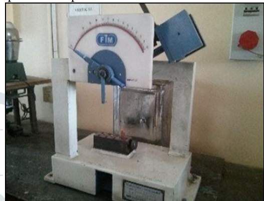
Fig. 10 Impact test setup
